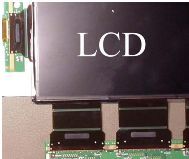
Figure 11 - Flex for FPD HDTV (Gilleo teardown)
