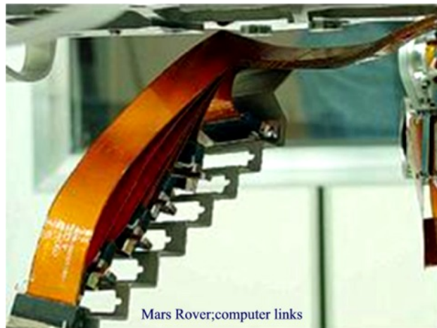
Figure 7 - Most Distant Flex? - Mars Rover
