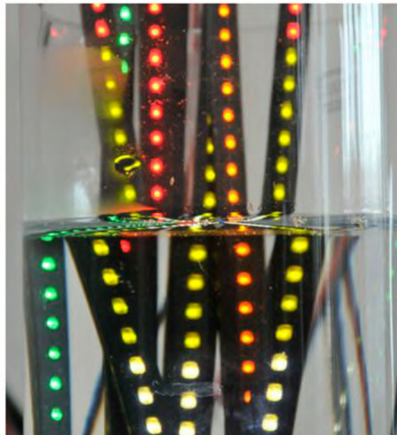
Figure 6: Device embedded components are resistant to any liquids that are resistant to standard PCB CCL based on epoxy resin.
