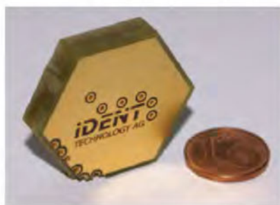
Figure 7: A sensor PCB with two layers of embedded components.
