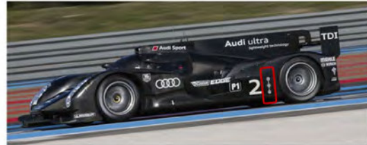
Figure 17: Embedded LEDs in racing cars reduce weight and improve functionality and safety.
