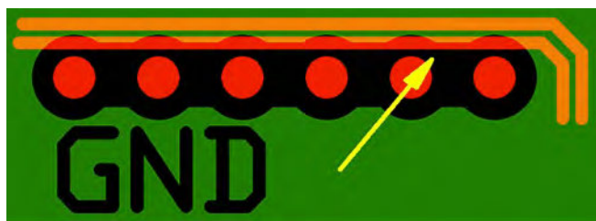
Figure 4: Unbalanced differential pairs due to too wide openings in GND plane and/or signals routed to close to pad.
