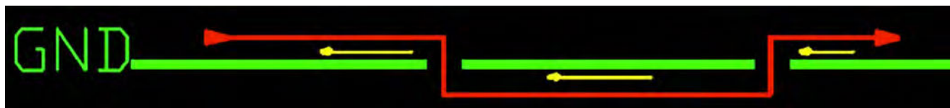
Figure 3: Return path shown in yellow. Reduced discontinuity if kept to same plane.
