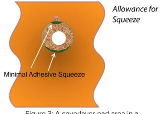
Figure 3: A coverlayer pad area in a Type 1, 2, or 3 application.
