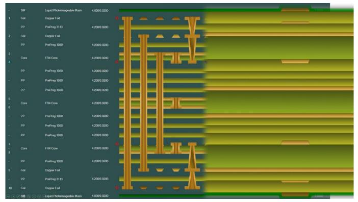
Figure 2: Side-by-side schematic and proportional view of the same stackup.
