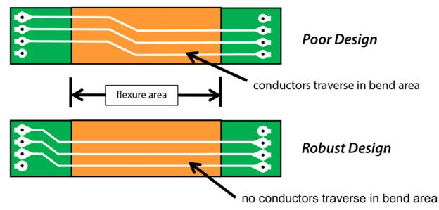
Figure 4: Note that the robust design is absolutely critical in flexing applications.
