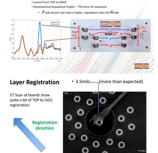
Figure 2: Effect of misregistration on differential escape (reproduced<sup>1</sup>).
