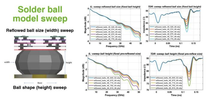
Figure 3: Effect of solder ball height on insertion loss and TDR profile (reproduced<sup>2</sup>).
