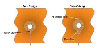
Figure 2: The example shows a cover-coated pad area in a Type 2 (double-sided) application.
