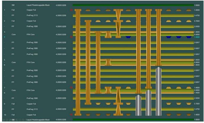
Figure 1: Schematic view of a stackup.
