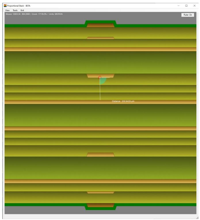
Figure 3: Proportional view expanded showing an isolation distance.
