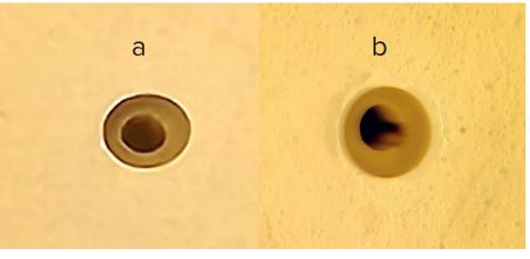
Figure 1: Photos of "good" and "bad" backdrilling.
