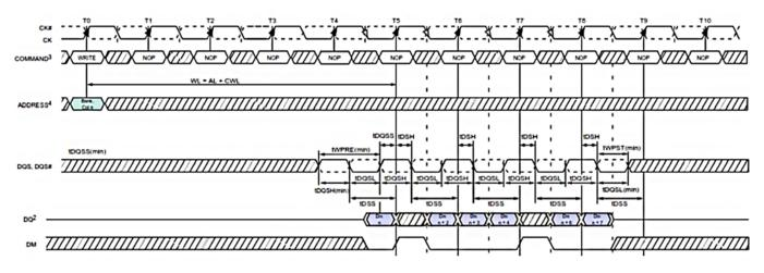
Figure 1: DDR3 synchronous timing. (Source: JEDEC Std 79-F3)
