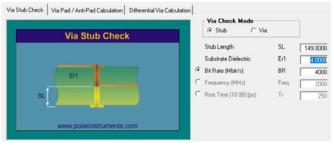
Figure 2: Via length of 149 mils causes some concern at 4 Gbit/s data rate.
