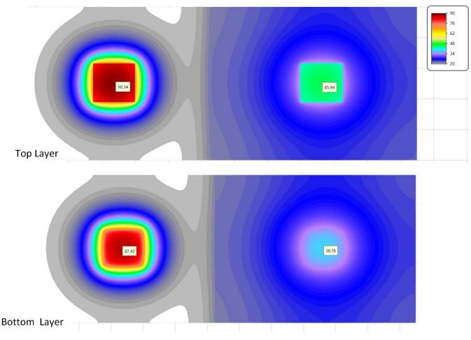
Figure 3: Heated pads, top and bottom layers.
