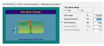
Figure 1: Via length of 28 mils causes no concern at 4 Gbit/s data rate.
