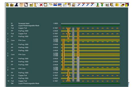
Figure 5: Stackup with microvia/back-drilled vias and buried vias. (Source: Polar Speedstack)
