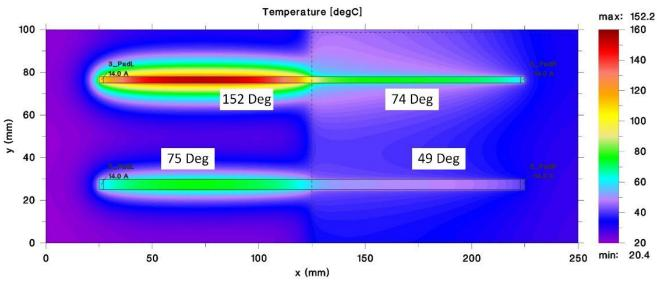
Figure 1: Planar impact on trace temperatures.
