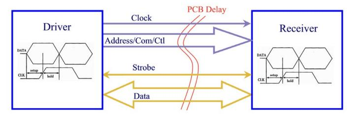
Figure 2: Source synchronous timing relationship across substrate.
