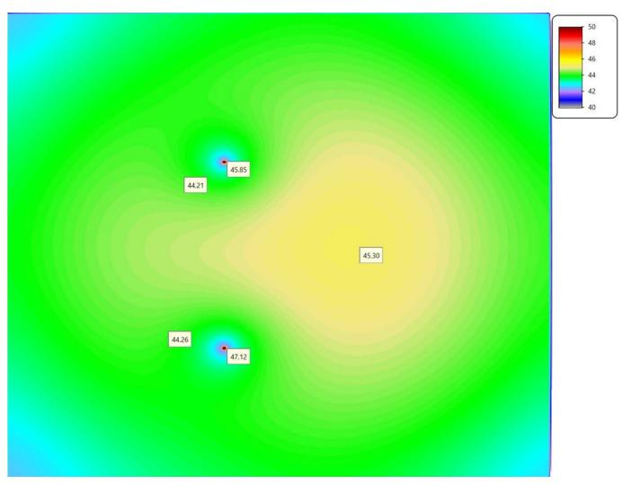
Figure 4: Thermal profile of top pad with two thermal vias.
