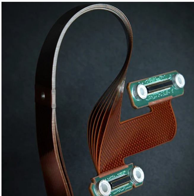
Figures 1 and 2: Mars Perseverance Rover utilizing extended length flex assemblies. (Source: Pioneer Circuits)
