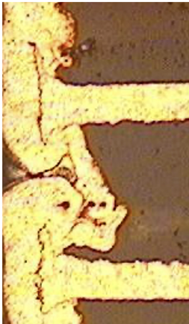
Figure 3: Poorly drilled plated through-hole with torn out glass and resin gouges.
