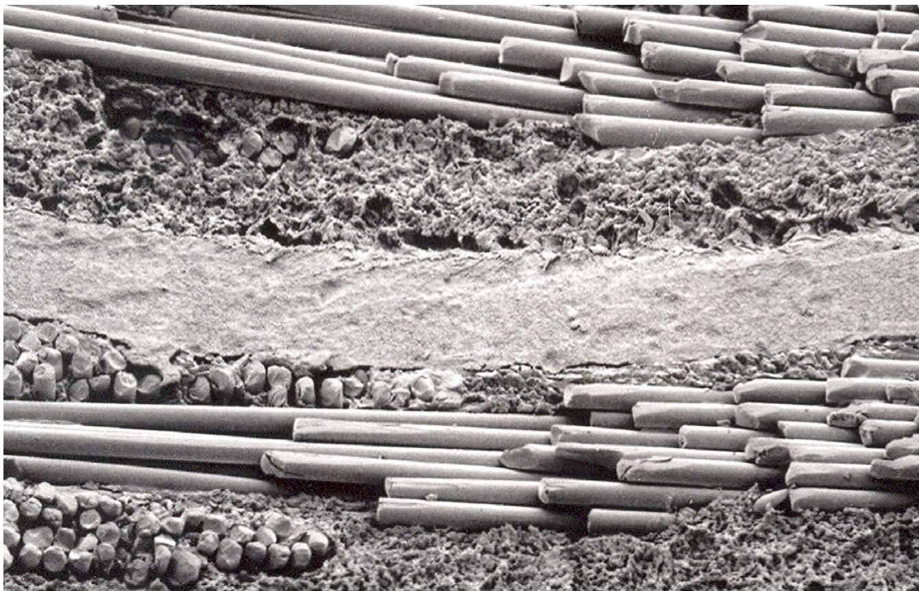
Figure 4: Desmear performance with microroughened texture to the resin.
