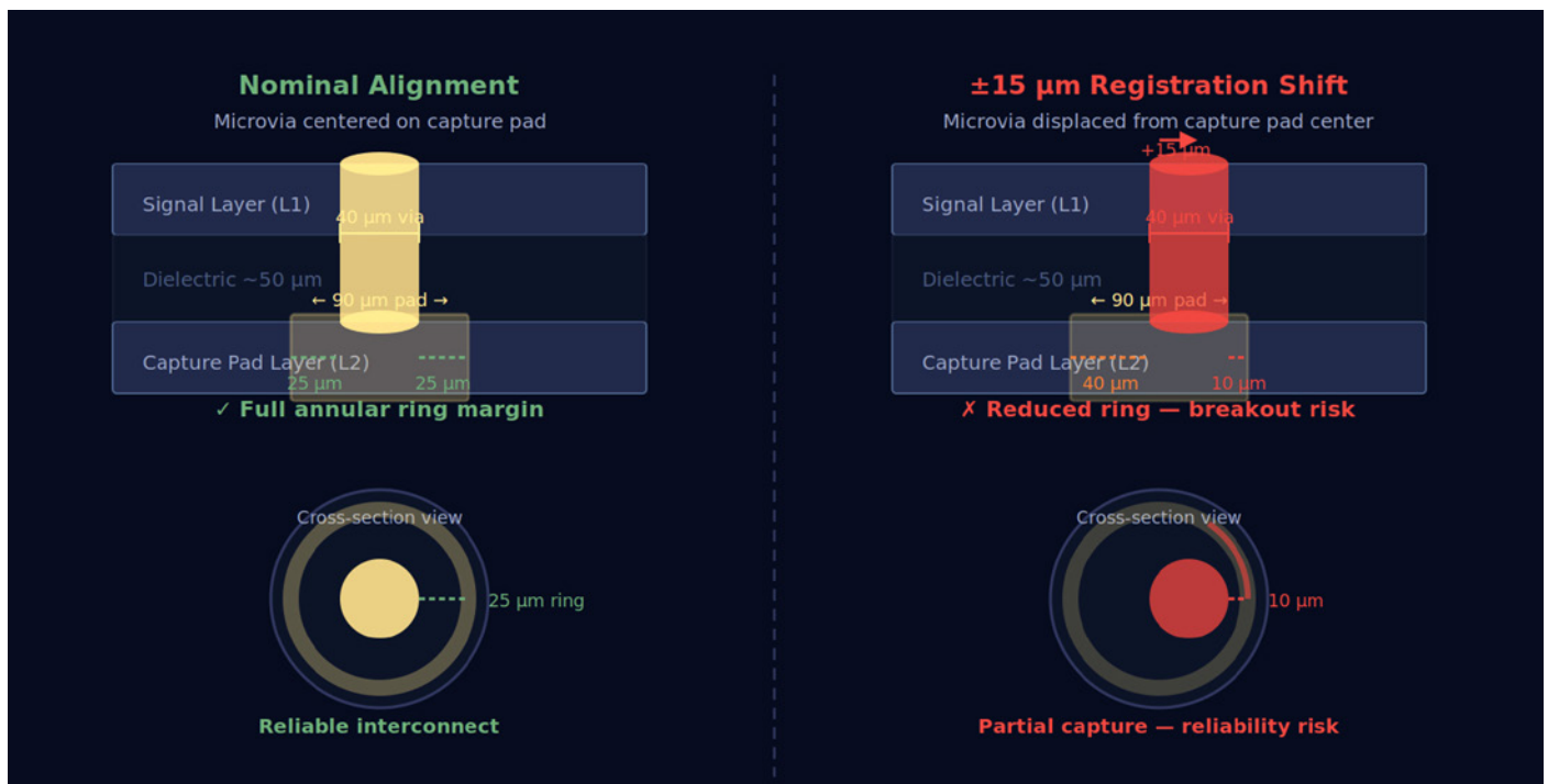
Figure 3: A 15\text{ }\mu\text{m} registration shift reduces capture pad annular ring from 25\text{ }\mu\text{m} to 10\text{ }\mu\text{m} , substantially increasing breakout risk. In ELIC, this condition exists at every level of the stack and compounds with each cycle.
