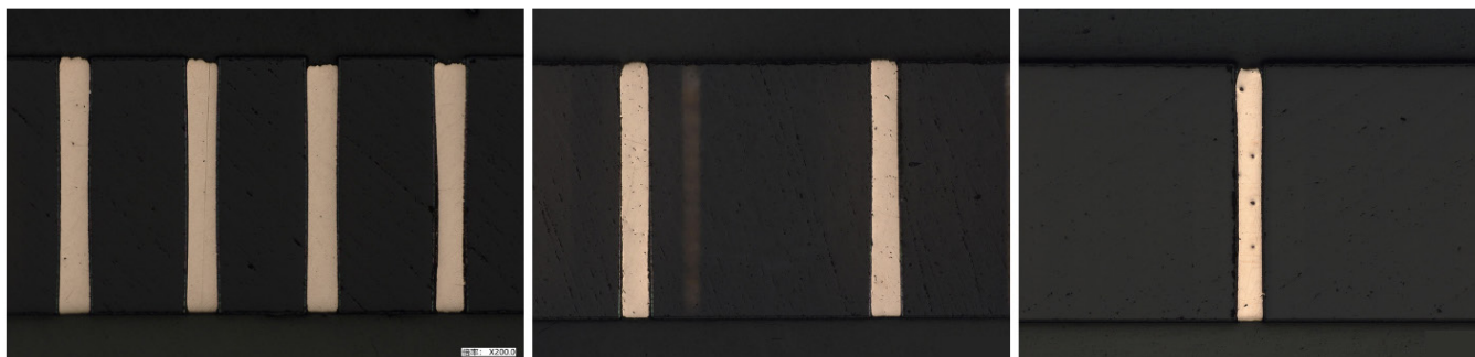
Figure 1: Cross-sections of through-glass vias (TGV) filled with bottom-top technology with different densities that show no voids.
