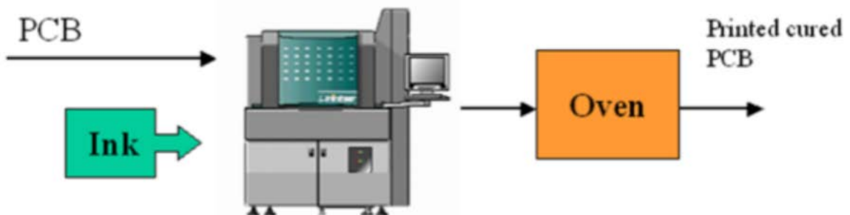
Figure 3: Process flow for legend print by inkjetting. (source: Printar)
