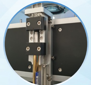
Automatic calibration using 50Ω airline
