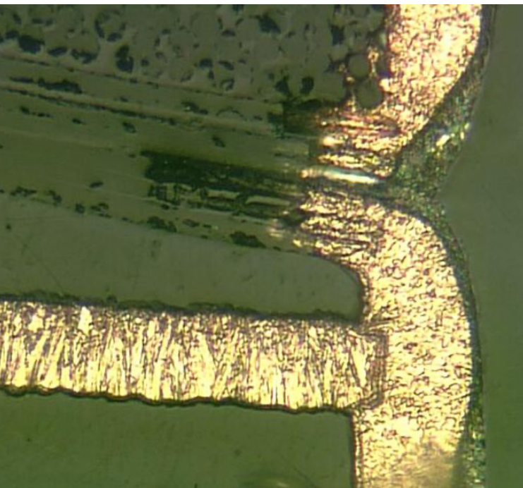
Figure 1: A rough hole wall, where glass fiber bundles were torn out exposing a deep gouge in the resin. Astonishingly, many feel the plating process should always compensate for such a travesty. A surface like the one shown here makes it very difficult to catalyze with the palladium-based activator from the electroless copper process.
