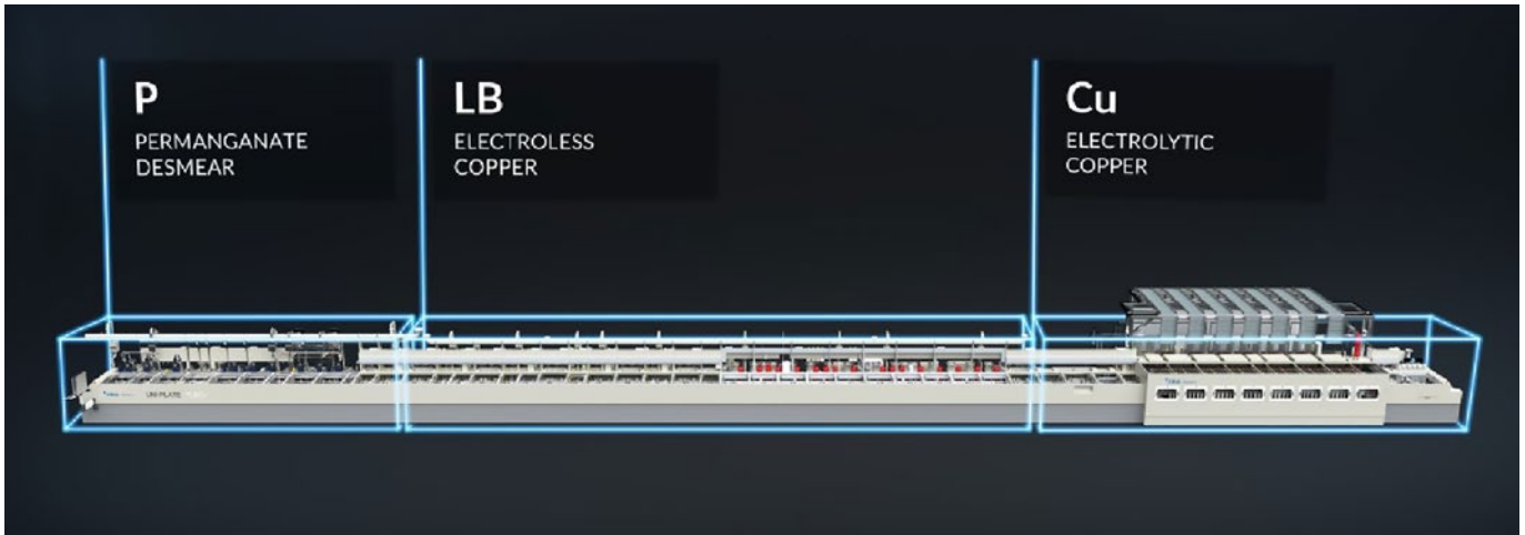
Figure 4: Uniplate® PLBCu6 for flash copper plating.
