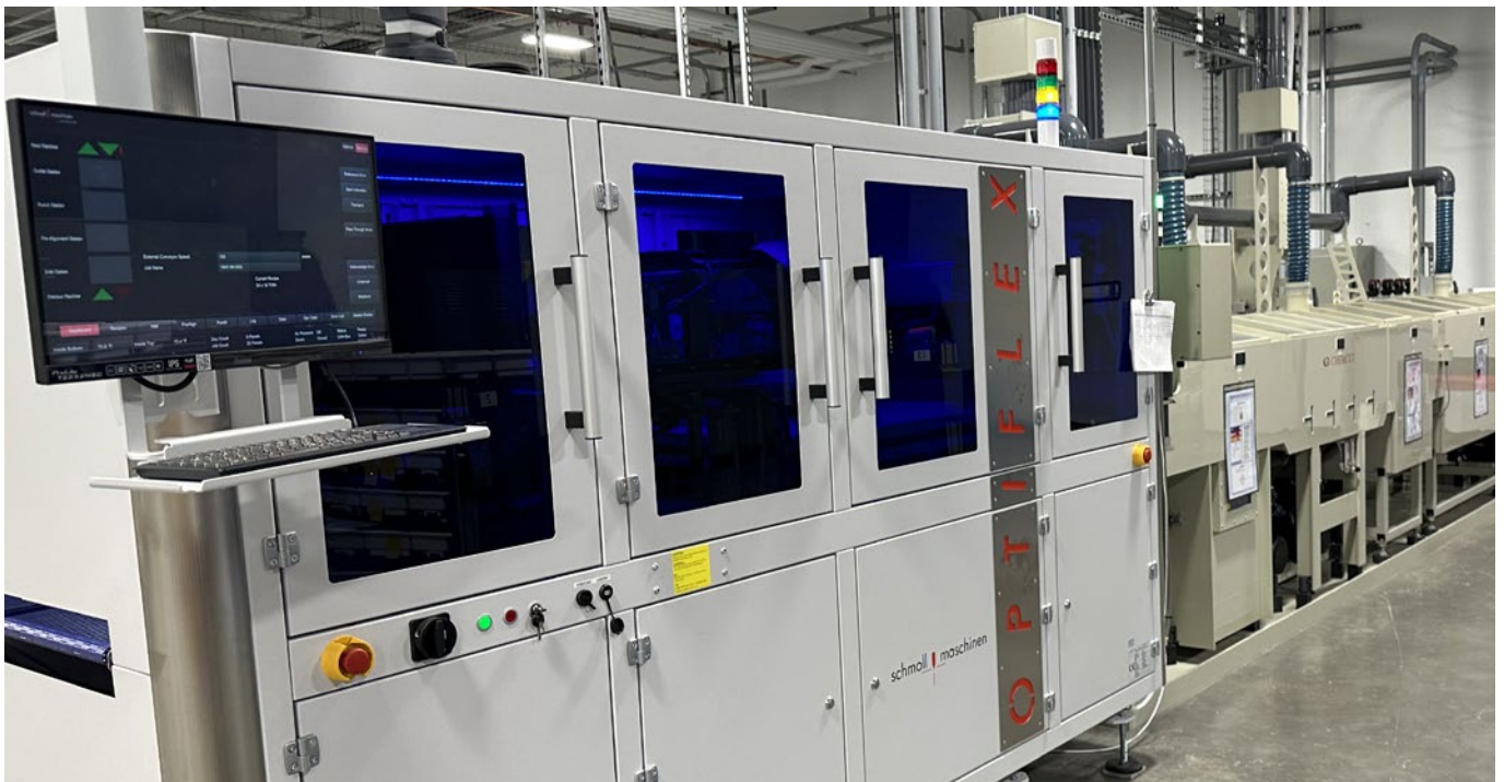
The highly accurate Schmolz Optiflex II post-etch punching machine.
