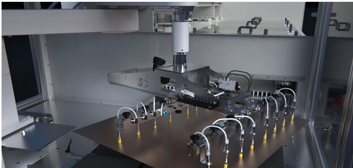
Figure 3: TGA system for 180° PCB turn/adjustment.
