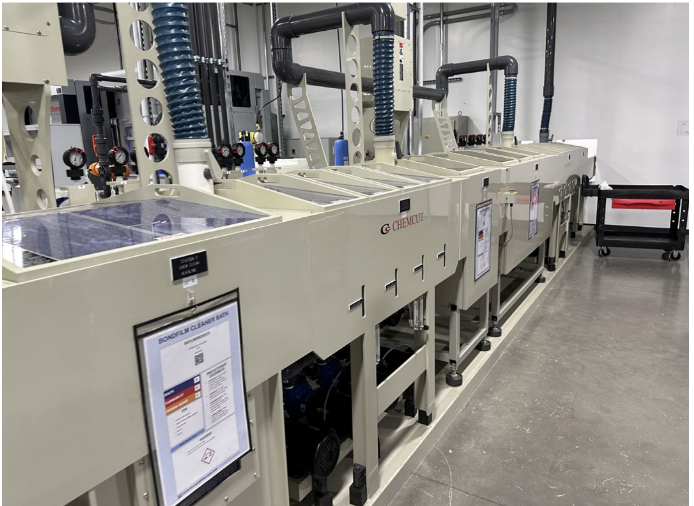
Chemcut chemical cleaning system.
