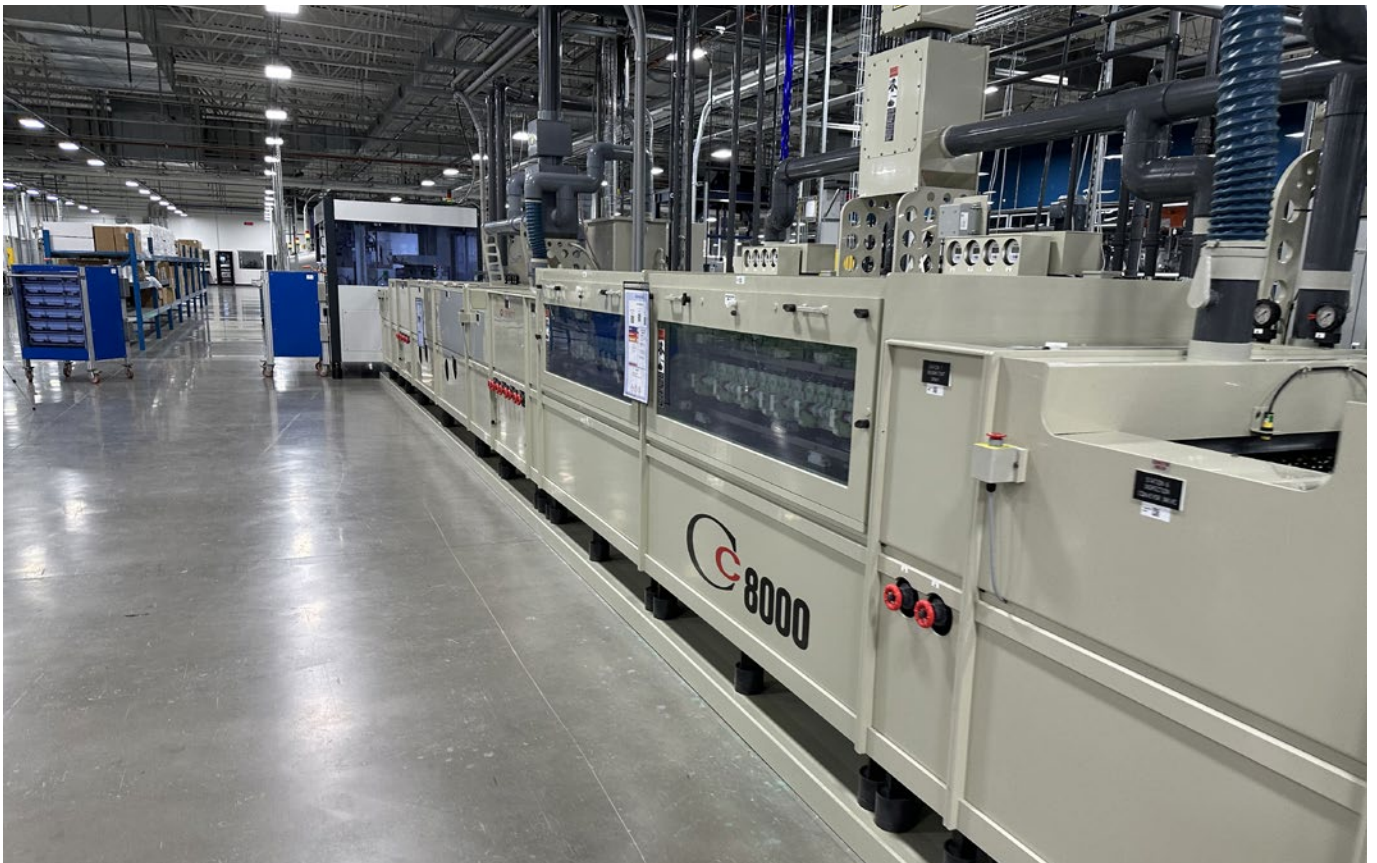
Chemcut CC8000 inner layer develop-etch-strip (DES) system using cupric chloride etchant. The two large portions of the line shown are the etching chambers.
