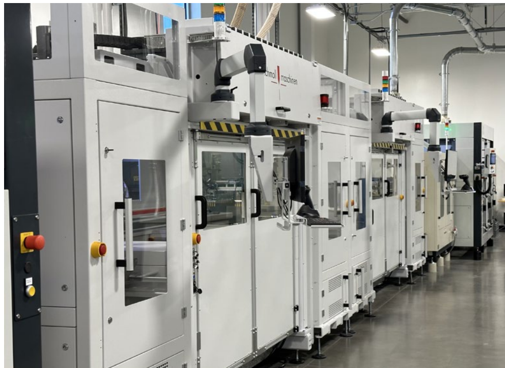
Positioned side-by-side, two fully-automated Schmolz XRA X-ray reference hole drilling machines.
