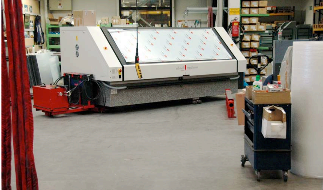
Fig. 12: A six spindle-drilling machine is rolling out of the factory. A radio controlled hydraulic roller movement systems takes the finished drilling or routing-machines that can weight up to 12 metric tons, out of the factory
