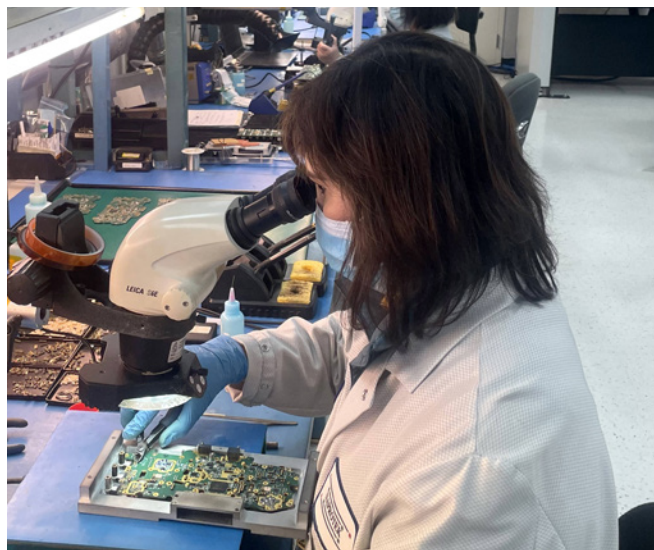
RF board under assembly.
