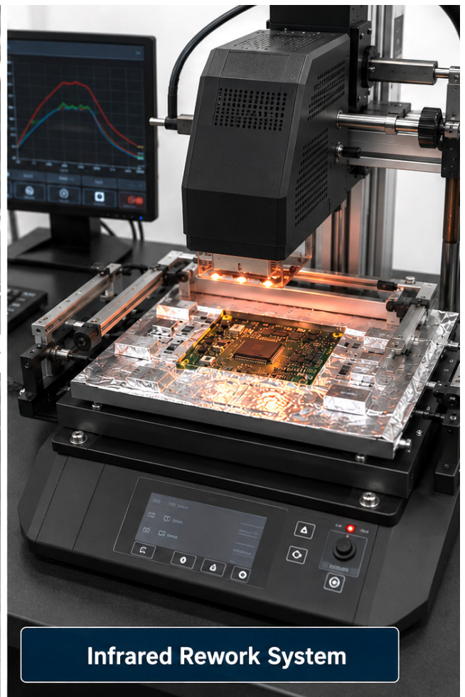
Figure 1: Hot air rework system and IR rework system for removal of electronic devices.
