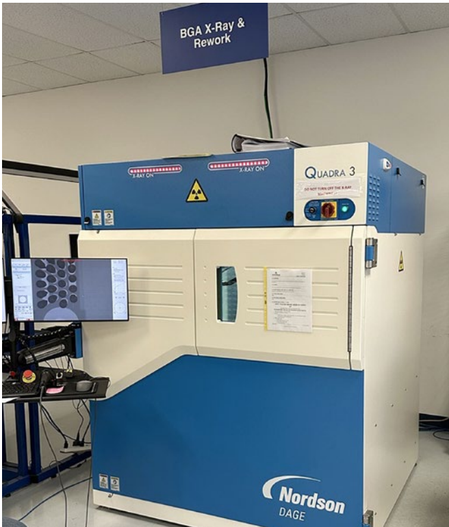
X-ray inspection system for production line quality control.
