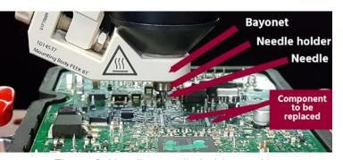
Figure 2: Needle, needle holder, and bayonet.
