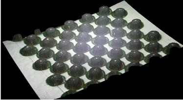
Figure 14: BGA component after jetting.
