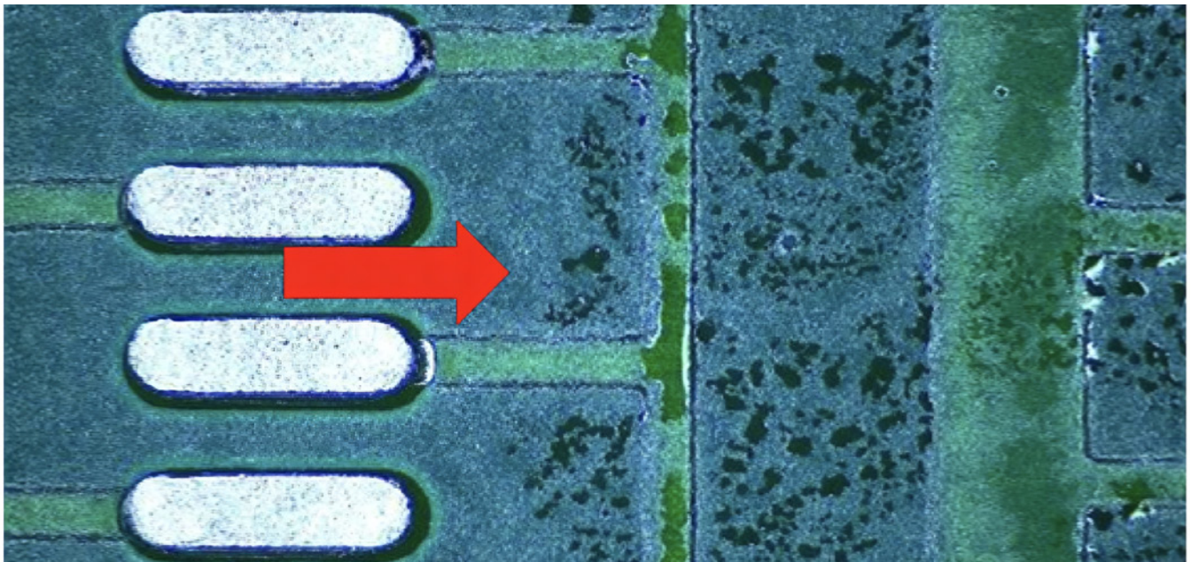
Figure 3: Example of poor rinsing beneath a low-standoff component.
