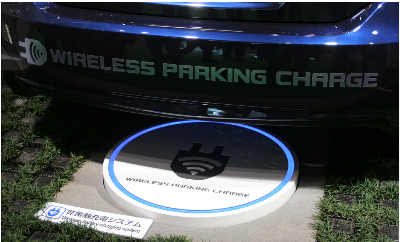
Figure 3: Induction wireless charger. (Source: Creative Commons, Neo, 2011)
