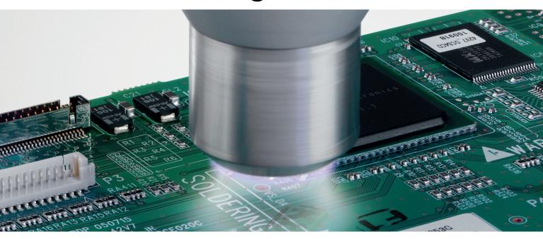
Openair-Plasma® offers potential-free, inline surface treatment and activation that can widen the process window to minimize waste and reach 100% yield.
