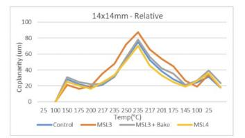
Figure 22: Average relative coplanarity, 14 x 14 mm (with outlier from Figure 18 removed from average).
