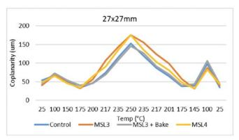
Figure 14: Average coplanarity over temp, 27 x 27 mm.
