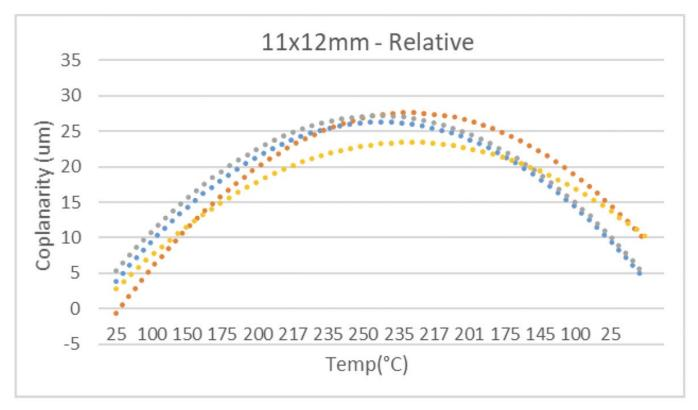
Figure 24: Average relative coplanarity, second-order polynomial fit, 11 x 12 mm.
