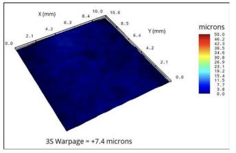
Figure 6: 10 x 11 mm, MSL3, 200°C cool down, low warp.
