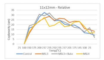
Figure 21: Average relative coplanarity, 11 x 12 mm.
