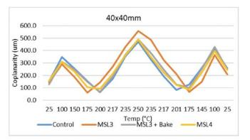
Figure 15: Average coplanarity over temp, 40 x 40 mm.
