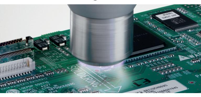
Openair-Plasma<sup>®</sup> offers potential-free, inline surface treatment and activation that can widen the process window to minimize waste and reach 100% yield.
