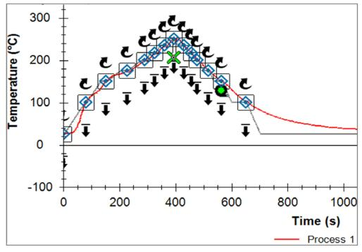
Figure 3: Example reflow profile output.
