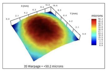
Figure 7: 10 x 11 mm, MSL4, 217°C heat-up, high warp.
