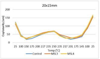
Figure 13: Average coplanarity over temp,  $20 \times 15$  mm.
