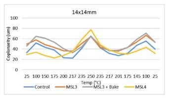
Figure 12: Average coplanarity over temp,  $14 \times 14 \text{ mm}$ .
