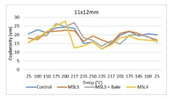
Figure 11: Average coplanarity over temp, 11 x 12 mm.
