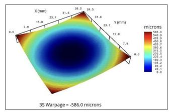
Figure 9: 40 x 40 mm, MSL3, 250°C peak, high warp.
