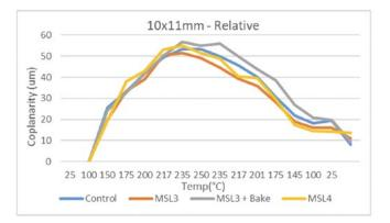
Figure 20: Average relative coplanarity, 10 x 11 mm.
