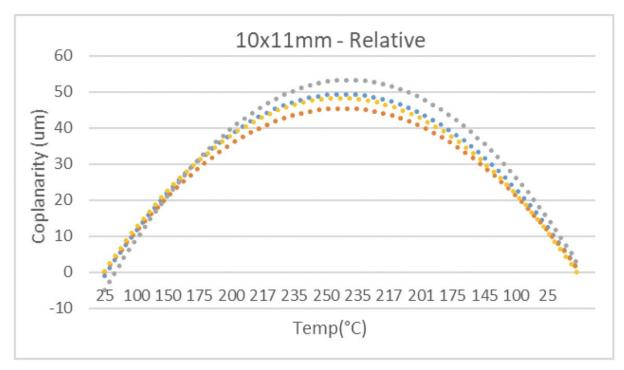
Figure 23: Average relative coplanarity, second-order polynomial fit, 10 x 11 mm.
