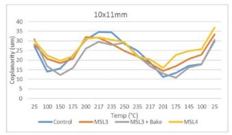
Figure 10: Average coplanarity over temp, 10 x 11 mm.
