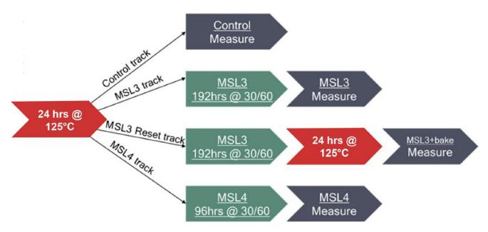
Figure 2: Moisture exposure tracks test samples.
