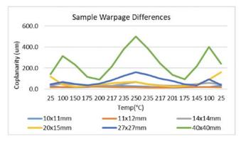
Figure 19: Overall coplanarity by sample size.
