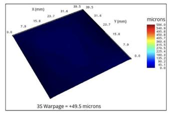
Figure 8: 40 x 40 mm, MSL3, 175°C heat-up, low warp.
