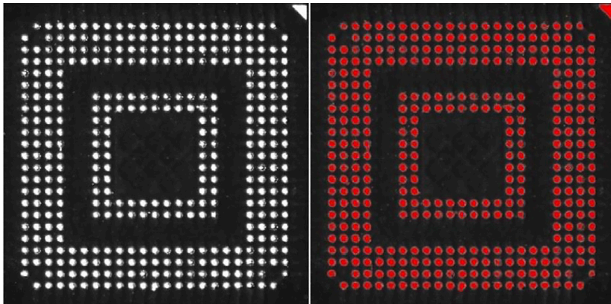
Figure 1: Masking by pixel saturation of solder balls on BGA 1.
